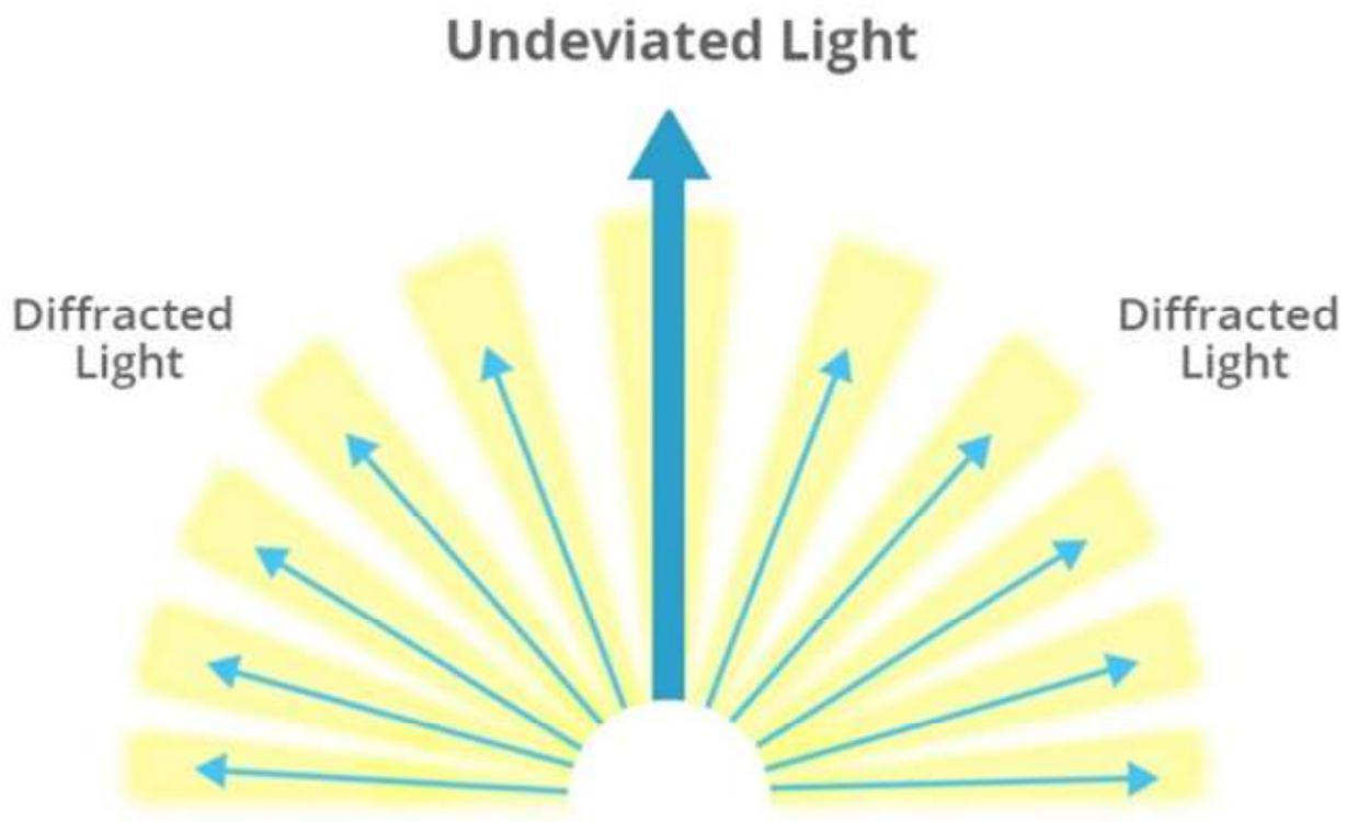
Light entering the camera from a single, small point has the potential to spread out at sharper angles, causing diffraction and softer images.
